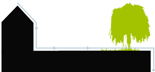
4.13 Rainwater bed Filtering runoff water from roofs before discharge into the harbour basin
